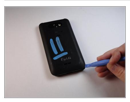
Use a plastic opening tool to remove the back cover.
