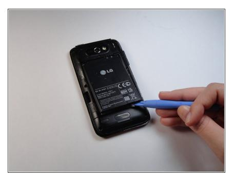
Use a plastic opening tool to remove the battery, lifting from the bottom right corner.
