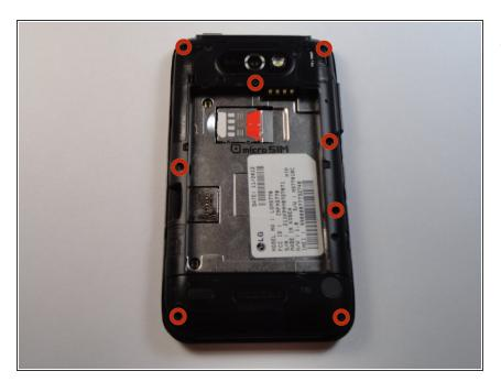
Use a Phillips #00 Screwdriver to remove all eight 4mm screws.
