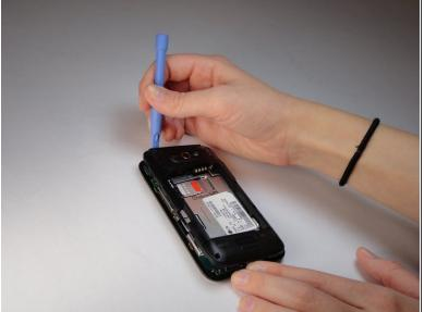
Use a plastic opening tool to remove the back trim by working around all of the edges.
