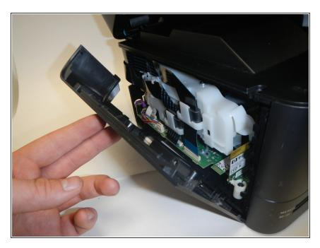
After unscrewing the screw, the left side will slide down revealing the wireless card.
