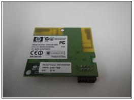
• Unscrew one 12mm screw and gently disconnect the wireless card from the motherboard.
