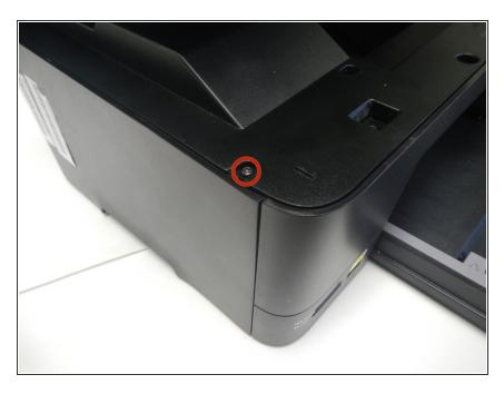
Using the T9 Torx Security screwdriver bit, unscrew the 12 mm screw on the far left side on the top of the printer.
