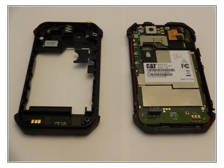
With all screws removed, the back and side pieces should come off the front of the phone, exposing the motherboard and various components as shown.
