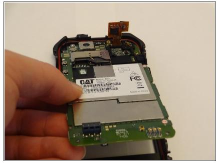
• Finally, disconnect the chip seen in the upper right, and the board should pull away from the rest of the phone.
