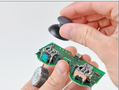
Pull both analog stick covers straight up off their joystick posts attached to the motherboard.
