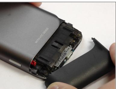
Apply pressure to the dark plastic casing and slide the casing downward, off of the phone.
