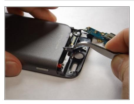
Once the back side of the buttons are exposed, they will fall out either by punching them out from the front side, or by using tweezers to pull them out of the back.
