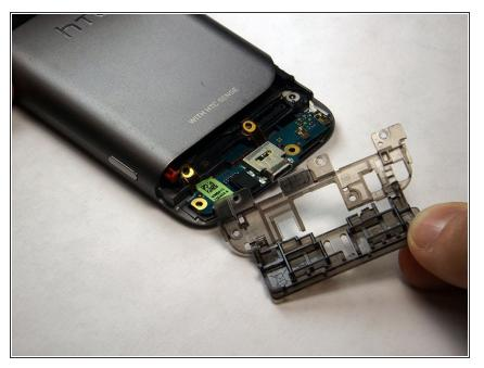
Once the screws are removed from the plastic flap, the piece should easily come out.
