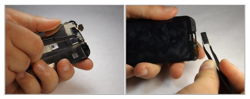
• The speaker should still be attached to the front of the phone, so push the speaker from the front, or use metal tweezers to grab and remove through the backside of the screen.
