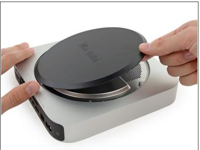
Lift and remove the bottom cover.
