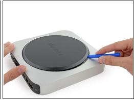
Use the plastic opening tool to pry the bottom cover up off of the Mac mini.
