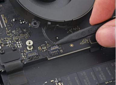
Use the point of a spudger to lift the fan connector straight up out of its socket on the logic board.
