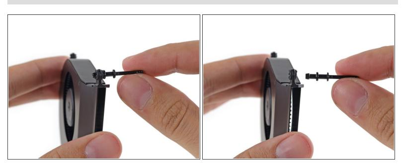
Remove the captive screw from the rubber grommet in the fan screw hole.
