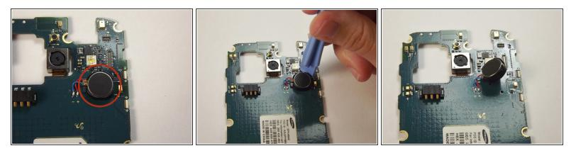
With plastic prying tool, lift up the vibration motor.
