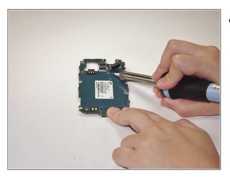
With the soldering iron remove the solder attaching the vibration motor to the motherboard.
