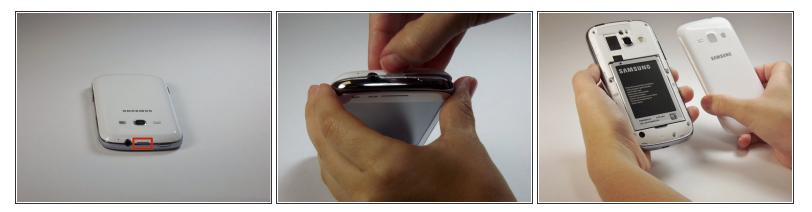
Using your finger nails or the spudger; pry the plastic casing open, and pull away from the body of the phone.
