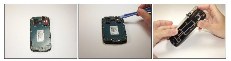
With the plastic prying tool, lift up the flap in order to fully open the motherboard.
