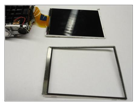
• The metal frame of the screen can be removed using a thin spatula or spudger. After the frame is removed the part of the ribbon connected to the screen is accessible.
