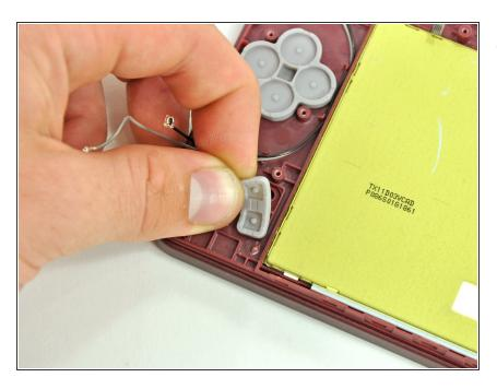
Lift the rubber pad off the back of the start/select buttons.
