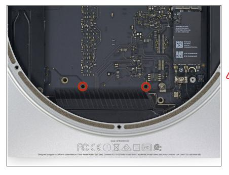
To remove the logic board, the two cylindrical rods of the Mac mini Logic Board Removal Tool must be inserted into the holes highlighted in red. Inserting instruments into any logic board holes other than the ones highlighted in red may destroy the logic board.
