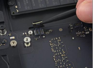
Use the flat end of a spudger to lift the SATA cable connector up off of its socket on the logic board.
