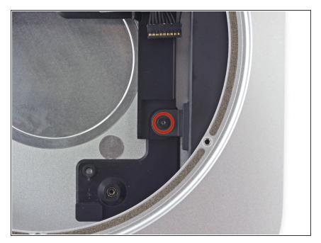
Remove the 8 mm T6 screw securing the power supply.
