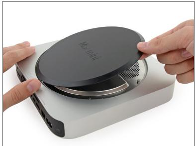
Lift and remove the bottom cover.
