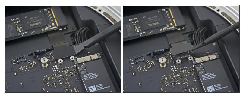
Lift the PCle SSD connector up off its socket.
