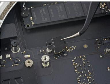
Remove the SATA cable connector bracket.
