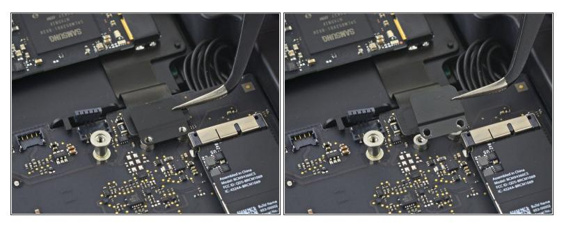
Remove the PCIe SSD cable bracket.
