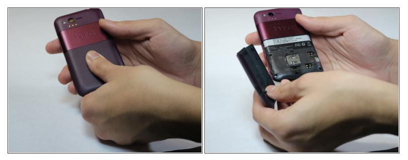
• Slide the bottom back casing off the phone.
