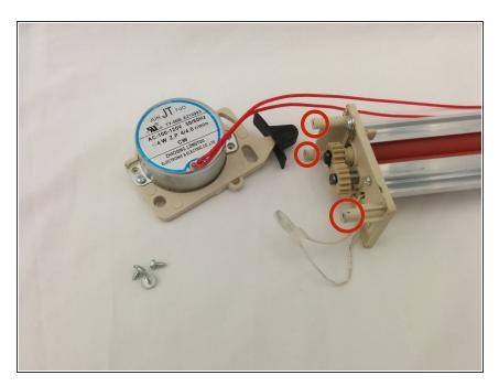
Remove the motor from the rollers by unscrewing the three screws holding them together.
