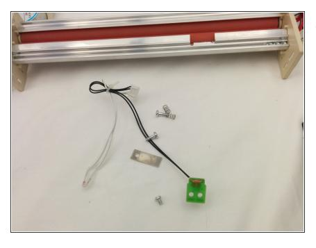
Remove the sensor from the roller enclosure by unscrewing the two spring-loaded screws.
