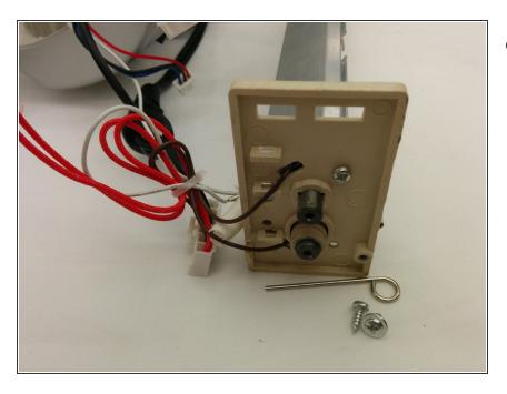
Unscrew the two screws and the bar on the other.
