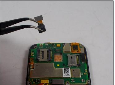
• Use a pair of <u>tweezers</u> to gently disconnect the camera connector and remove the rear facing camera.
