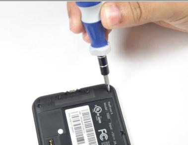
• Remove the thirteen 3.6 mm screws using the torx T5 bit in the screwdriver.
