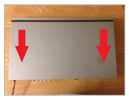
to remove the cover of the device, pull the cover towards the back of the device until it is completely removed so you can see the insides of the device
