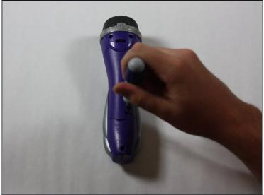
• Remove the back panel of the device by unscrewing the single #8 1<u>1.6 mm Flathead</u> screw on the back of the device.
