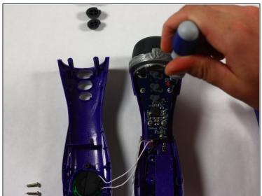
• Remove the 2, #8 11.7 mm Phillips Head screws as well as the 2, #8 7.5 mm screws on the printed circuit board.
