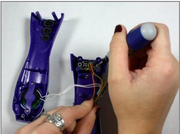
Remove the 2, #8 11.7 mm Phillips Head screws on the On/Off Switch Board
