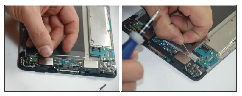
• Disconnect the thin connector wire. Note the position both ends go to. There is a similar connection at one end of the wire that could be confused for the correct connection. Incorrectly reconnecting the wire upon re-assembly to this terminal will result in a malfunctioning unit!
