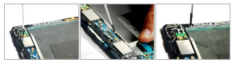
• Remove the 4 screws securing the motherboard.
