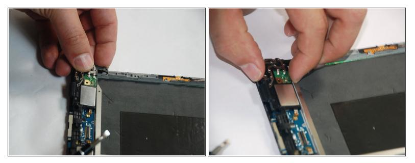
• Replace the original motherboard with the new circuit board.
