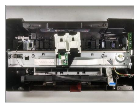
• Lift the metal structure from the printer, which will include the ink cartridge holders.
