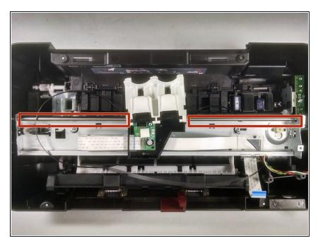
• Locate the metal bar that will be running parallel to the metal structure that was just removed. Locate the washer at one end.
