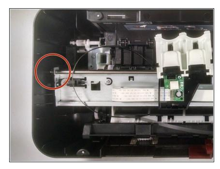
• Use the tweezers to pry off the washer, then slide the belt out. Lift the ink cartridge holder from the metal piece, separating the two.
