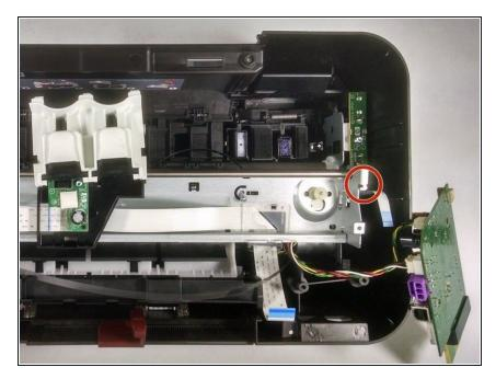
On the right side of the printer there will also be a spring. Again, disconnect this spring using the tweezers.
