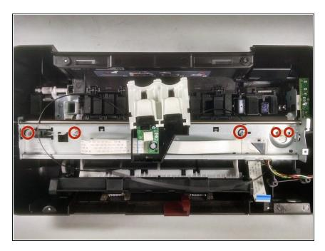
Unscrew the screws that are holding the metal structure in place. This includes the screw that is on the right side near the wheel the carriage driver belt was around. Be sure to note the size of the screws and where they go.
