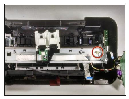
• Push the ink cartridge to the center of the printer so that the wheel on the opposite side is visible. Then lift the belt from that wheel.
