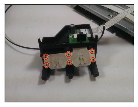
• On the front portion, detach the white paper from the holder. There will be six tabs that can be pushed though the paper to do this.
