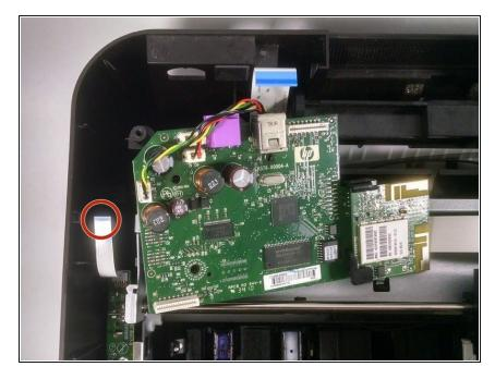
• Pull the narrower cord out of its connection, holding the blue-sealed end.
