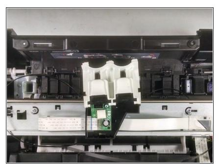
• Locate the white, ink cartridge holder. Find the three connections to the black part, this will be towards the base where the white paper is.
