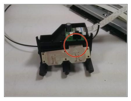
• Thread the white paper through the whole so that the latch holding the cartridge belt is visible.
