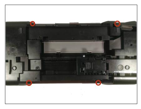
• Turn the printer upside down. Locate the four screws holding the cover in place. These will be on the edges of the cover.
