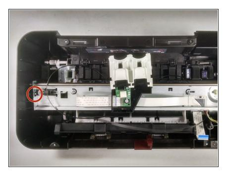
On the left side, between the wall of the printer and the metal piece, there will be a spring connecting the two. Use the tweezers to detach the spring and keep separate.
