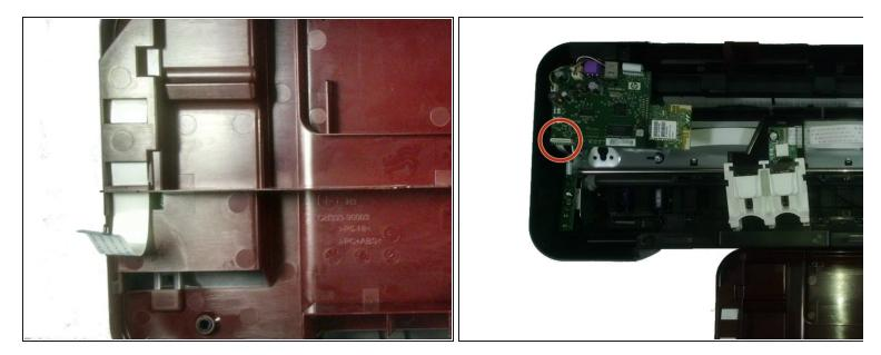
• Detach the wire from the printer by pulling the blue-sealed end from the white holder.
