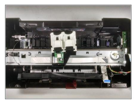
• Pull the belt tightly to this side, creating enough slack to lift the belt from the wheel.
