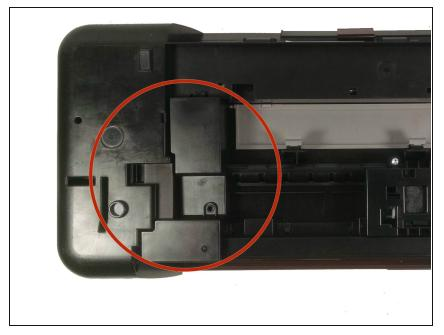
Flip the printer upside down and locate the cover on the left hand side. It is rectangular shape and is held in place by two screws. Unscrew these screws and take off cover.
