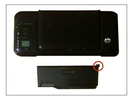
• To release the tray from the printer, you must manually pull it out. Hold the tray and push towards one side of the printer. Then pull away from the printer towards the other side. Keep output tray separate.
