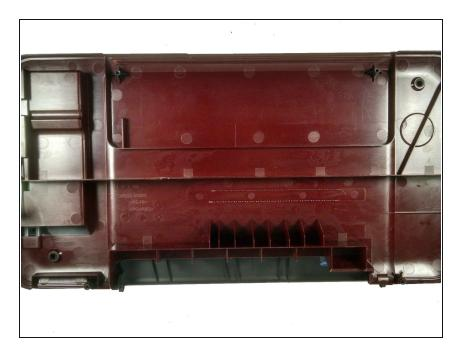
Place fingers on the edge of the red cover. Begin to pull upwards to release the top portion, working your way around the printer. Make sure that it does not fall back into place.
