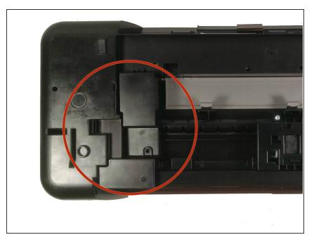
Flip the printer upside down and locate the cover on the left hand side. It is rectangular shape and is
