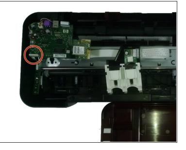
Detach the wire from the printer by pulling the blue-sealed end from the white holder.
