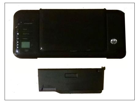
Begin to disassemble the printer by disconnecting from all power sources and computers. Keep cords separate and allow the printer to cool for 5 minutes.
