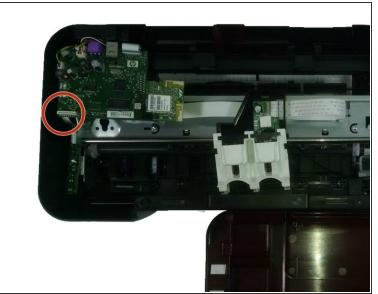
Once the top is loose, there will still be a connection wire between the printer and the cover. This
