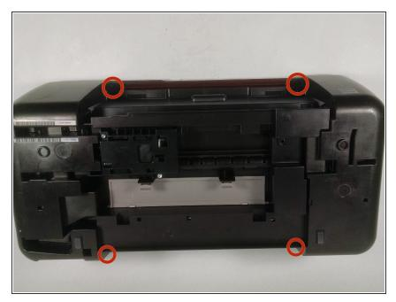
Unscrew the four screws, keeping them separate. Turn the printer back right side up
