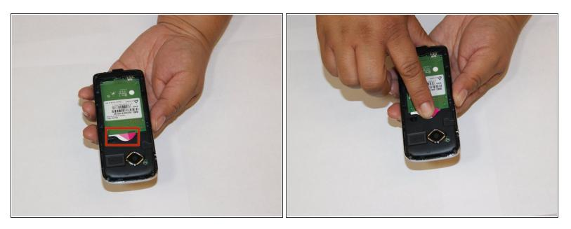
• Remove the SIM card by placing your index finger over it and sliding it out.
