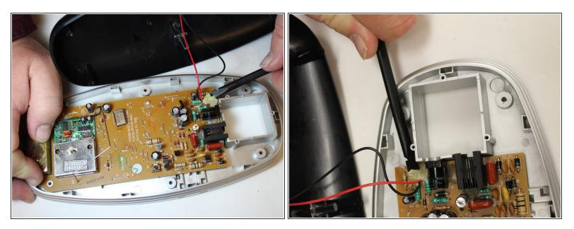
Use the spudger tool to carefully scrape the glue off of the connection points of both the black and red wires.
