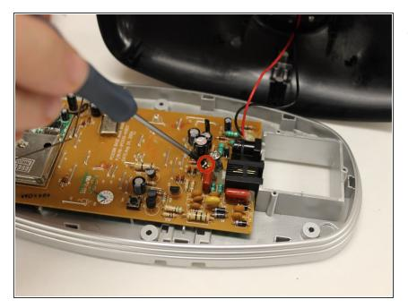
Use a Philips #00 screwdriver to remove the single 6mm screw from the motherboard.
