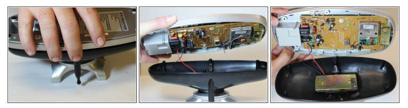
• With the base turned upside down, grasp the edges of the base plate and gently lift from the rest of the base.
