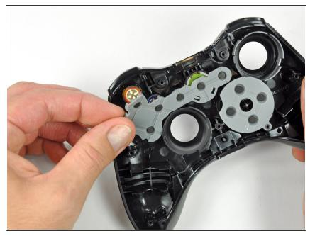
• Remove the rubber pad from the back of the input buttons.
