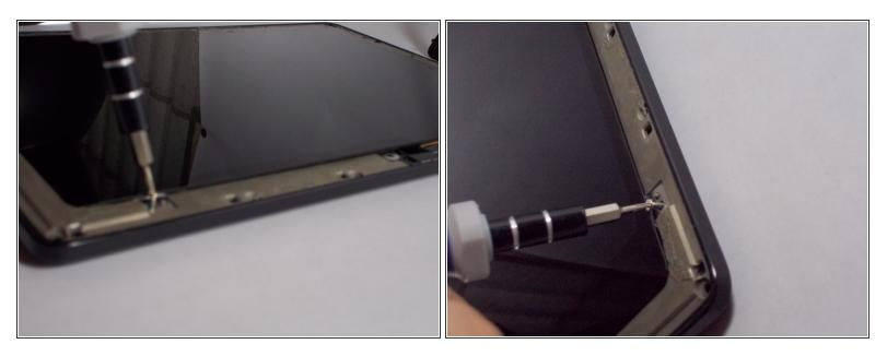
Remove every visible screw from the front of the nook using the T-4 attachment for the screwdriver in the iFixit screwdriver kit.
