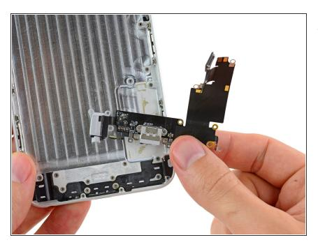
Lift and remove the Lightning connector and headphone jack cable assembly out of the iPhone.
