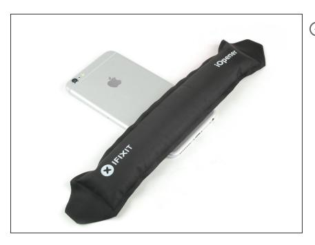
The next step requires peeling up the Lightning connector and headphone jack cable that is affixed to the inside of the rear case with mild adhesive. We highly recommend using an iOpener on the lower backside of the rear case to soften the adhesive.
