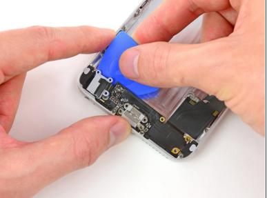
Run the opening pick across the top of Lightning connector and headphone jack cable to loosen the adhesive securing it to the rear case.
