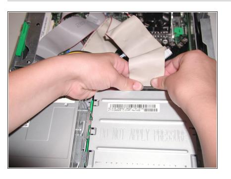
Pull Ribbon Cable Straight Back, and Out of Cd drive Using the Plastic Tab.
