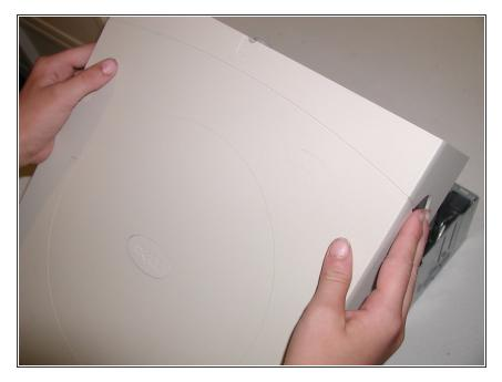
pull cover UP while holding in the 2 buttons on either side of the optiplex.
