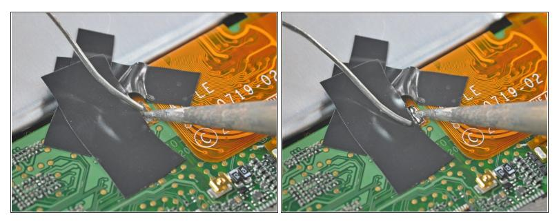
• Place your battery in the rear panel, with the **cable side down**, and use two small strips of electrical tape to hold the cable against the solder pads.
