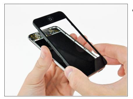
Lift the front panel out of the rear case minding the cable still attaching it near the upper left corner of the Touch.
