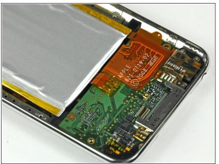
Don't forget to reapply the piece of tape over the solder pads to prevent any shorts.
