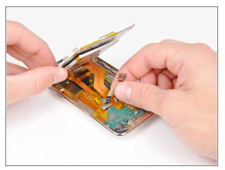
Peel the display data cable off the adhesive securing it to the rear panel.
