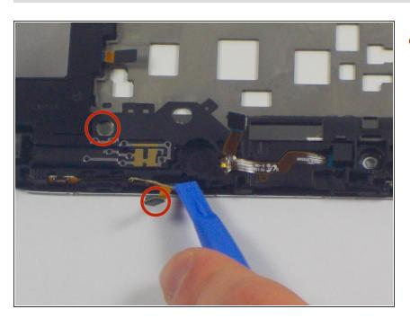
Using the plastic opening tool, gently detach the volume buttons cable from the motherboard by prying its connector upward.
