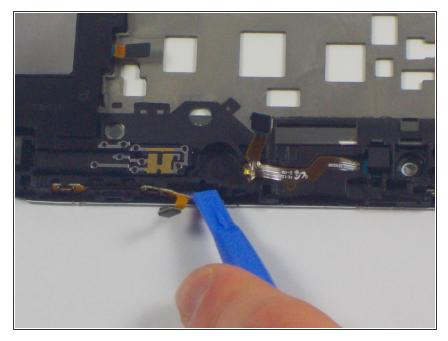
• Insert the plastic opening tool in between the volume buttons and the inner framework. Gently slide the opening tool to the left, releasing the volume buttons from the framework.
