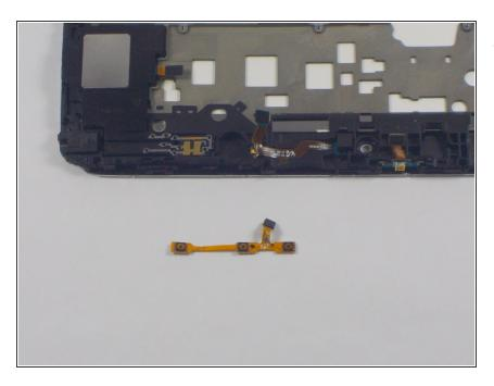
Gently remove the faulty buttons and insert new buttons. Be sure to properly attach the buttons to the motherboard via its cable.
