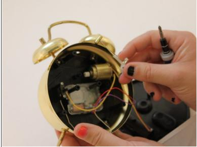
Using a Phillips Screwdriver, remove bell from inner clock.
