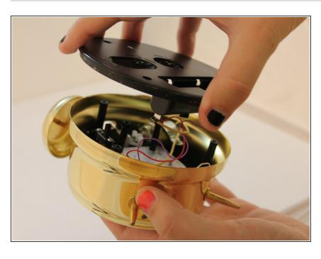
Place fingers on ridge around back plate and pull upward.
