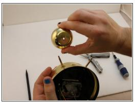
After you remove the screws for both bells, both of the two bells and the bar connecting the two bells will easily come off. Remove these three components with your fingers.
