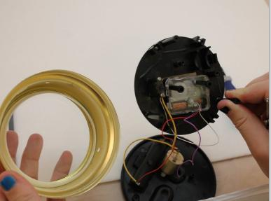
Using your hand, remove the entire black, inner apparatus of clock. The golden ridge of the clock is attached to the glass screen.
