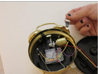
Using a Phillips screwdriver, remove the silver base located on top of cellinoid in upper right hand of inner clock.
