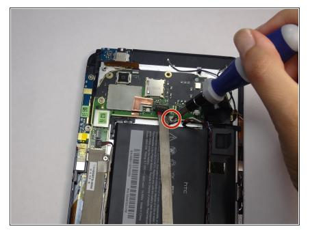
Remove the single 2.5mm Torx T5 screw holding the battery down along the top side.
