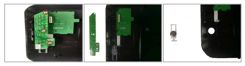
Unscrew the three screws indicated in the image. Unplug the connection from the screen, lift up the board, and remove from the panel. Pull the button out.
