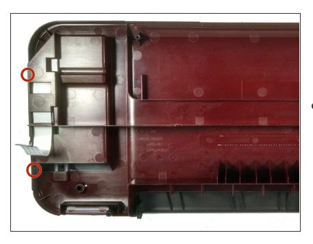
The control panel is connected to the maroon panel by four plastic hooks (two are seen in the picture and the other two are opposite them). Using a plastic opening tool pry each hook out of its locked position.
