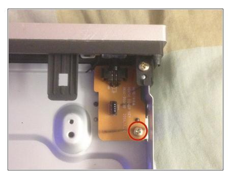
Unscrew the one screw that is connecting the circuit board to the frame.
