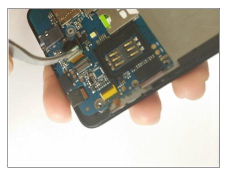
• Remove the ribbon cable next to the camera carefully.
