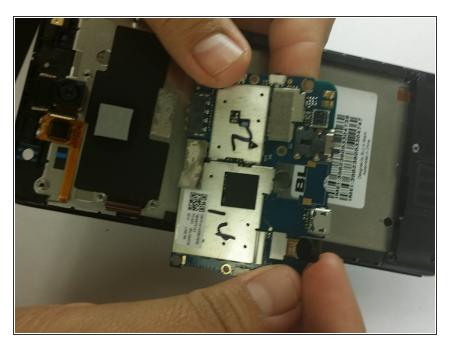
• Remove the motherboard of the phone and replace camera.
