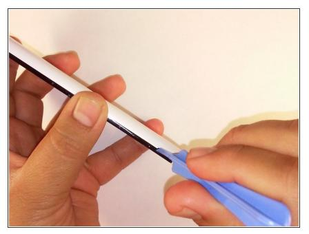
• Remove the back cover of phone with the plastic opening tool.
