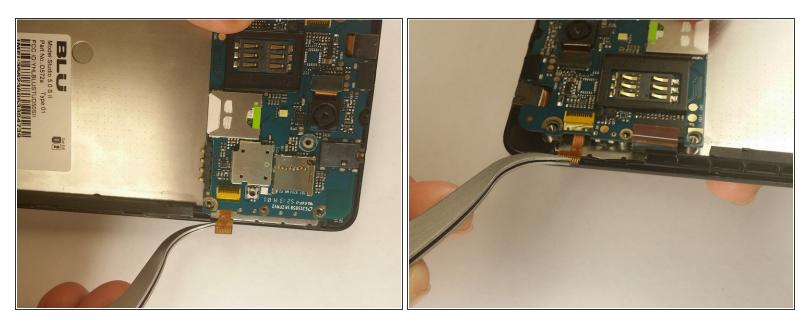
• Remove the ribbon cable carefully on all four sides of the motherboard of the phone.
