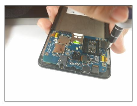
• Take off the four interior screws that are on the motherboard of the phone.
