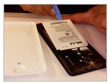
• Remove the battery with the plastic opening tool.
