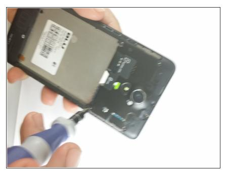
• Use the Philips #00 screwdriver to remove the nine screws that the top back part of the phone has.
