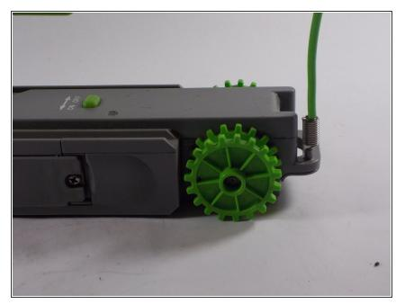
To remove the wheel simply unscrew the screw in the center of the wheel
