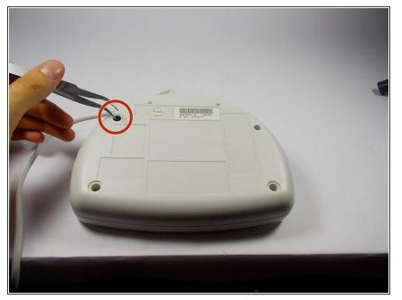
Begin by looking at the bottom face of the device. Use the tweezers to remove the four foam pads which are covering four screws
