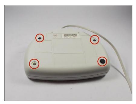
• Use the #2 philips screwdriver to remove the four screws from the bottoms of the device. These screw heads are sized 5.3mm or .209 in
