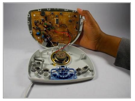
Remove the back casing panel by gently pulling back until you are able to reach the inside. gently pull the microphone out of its housing. This is only held in by friction so its easy to remove
