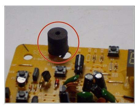
Pull out the old microphone and discard it the correct way. Place the new microphone in the same spot
