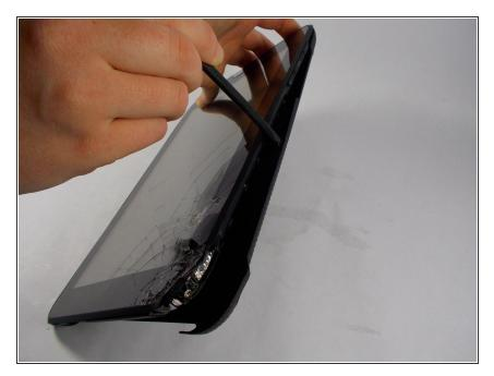
To remove the outer casing, wedge the pry tool in between the front and back panel, and pull them apart.
