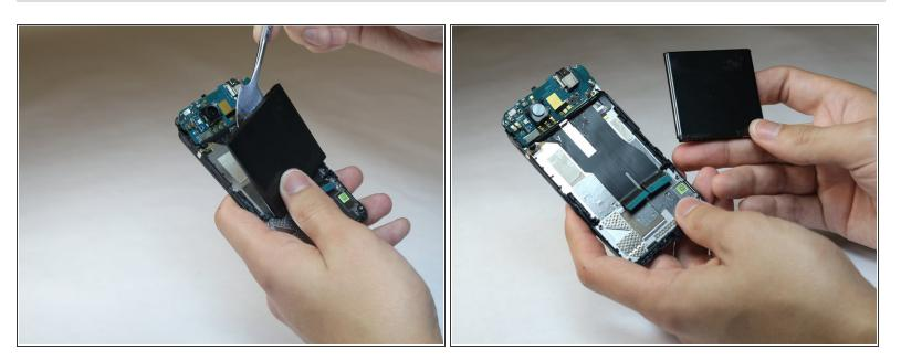
Using the metal spudger, remove the battery from the base.
