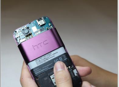
Using the plastic tool, pry underneath the top plastic cover.
