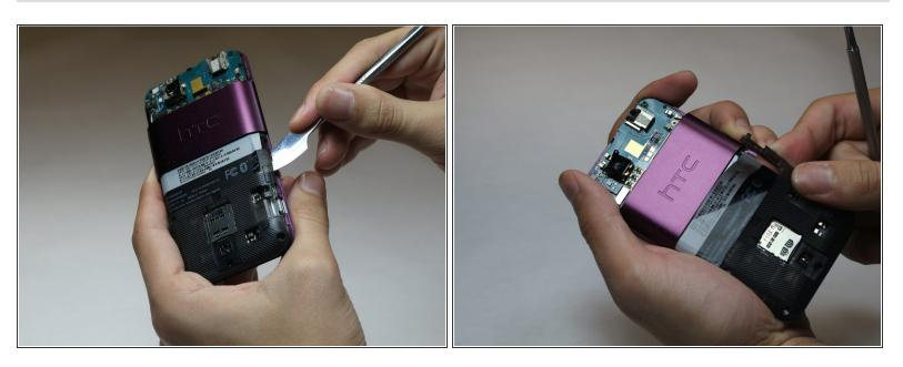
Using a metal spudger, pry up the plastic piece covering the motherboard, and remove the sticker.
