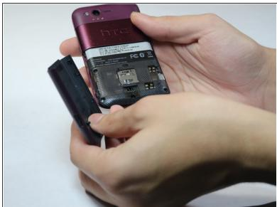
Slide the bottom back casing off, pulling down.
