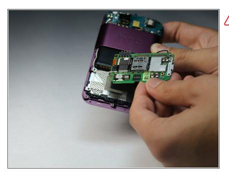
Carefully remove the motherboard from the base of the phone.
