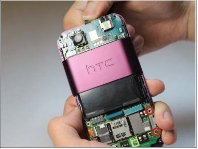
• Using a Phillips #00 screwdriver, unscrew the four screws in each corner of the motherboard.
