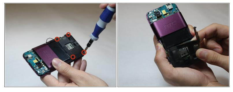
• Use a Philip #0 screwdriver to remove the four screws of the plastic covering the motherboard.
