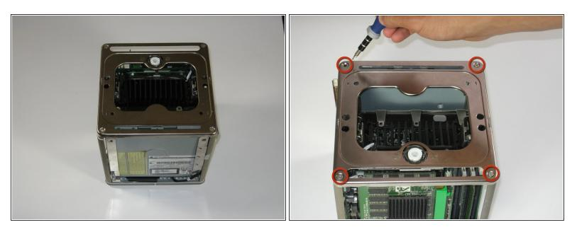
Place the cube upside down and remove the four T10 Torx screws on the front plate. Then remove the two screws on each side.
