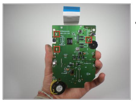
Disengage the the three plastic clips that secure the screen to the circuit board.
