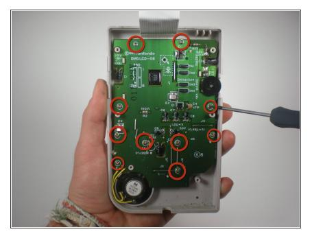
• Remove the ten screws that connect the circuit board to the outer case.
