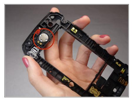
Locate the speaker on the back of the midframe.
