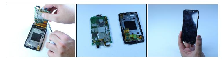
• Carefully use the <u>tweezers</u> to separate the motherboard from the screen.
