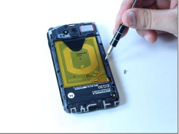
• Use the T5 screw head to unscrew the 9 silver screws from the housing frame. Carefully separate the housing frame from the motherboard.
