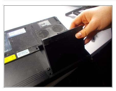
Just lift the battery up and out, making sure to lift from the end near the latch.
