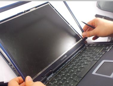
To finish removing the cover, grab the corners near the hinges and gently lift out, up, and away from the hinges.
