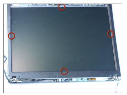
Using a fingernail or opening tool, gently pry the bezel up from the screen.
