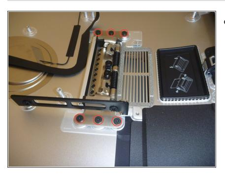
Remove the six screws holding the stand to the iMac back.
