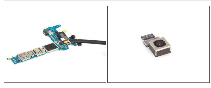
By the way, remove rear camera from motherboard. Release the connector and can take the camera away easily.
