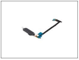
Release navigation button flex connector ,get it free from the adhesive on the mid-plate and remove it.
