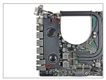
Remove the two 7.9 mm Phillips screws securing the left speaker assembly to the logic board.
