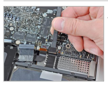
Use the flat end of a spudger to lift the hard drive cable connector up and out of its socket on the logic board.
