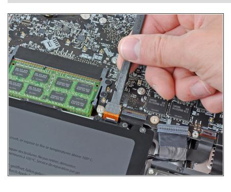
Use the flat end of a spudger to pry the trackpad connector up and out of its socket on the logic board.
