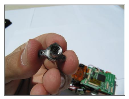
Remove the tripod mount from the bottom of the camera and set it aside.
