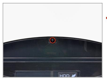
Remove the single 8.5 mm T10 Security Torx screw from the smart plate.
