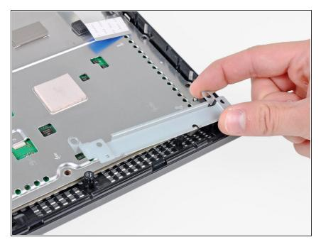
• Remove the control board bracket.
