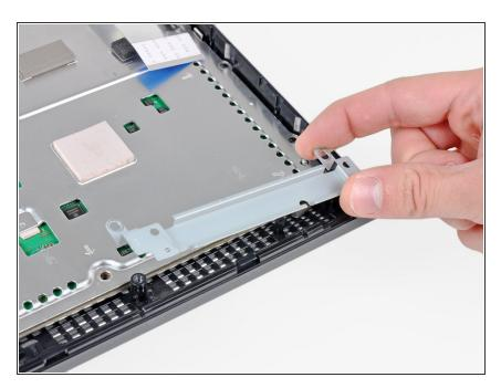
Remove the control board bracket.
