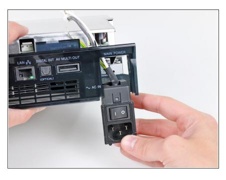
Pull the AC inlet out from the bottom of the rear cover, minding any of its cables that may get caught. To reassemble your device, follow these instructions in reverse order.
