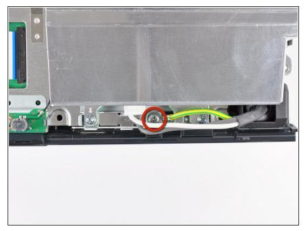
Remove the 7.7 mm Phillips screw securing the ground strap to the chassis.
