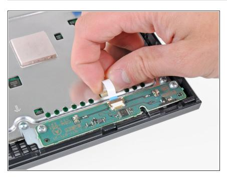
Pull the control board ribbon cable straight up and out of its socket on the motherboard.
