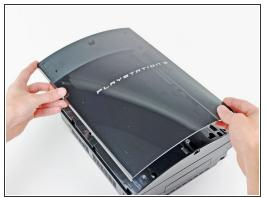
Pull the smart plate toward the hard drive bay, then lift it off the body of the PS3.
